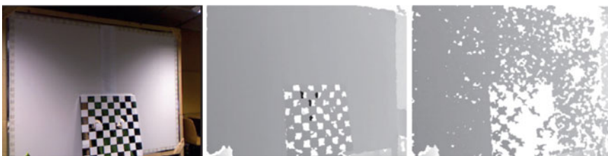
Fig. 2.1 A simple scene ( left ) captured with the depth camera of one ( middle ) and multiple concurrently projecting kinects ( right ). The interference of more than one Kinect pattern results in degradations in the captured depth image ( white pixels denote invalid depth values). This state of the art report lists significant papers that implemented setups albeit interference issues or to specifically address and overcome these issues. Reproduced from Schroeder et al. [44]
