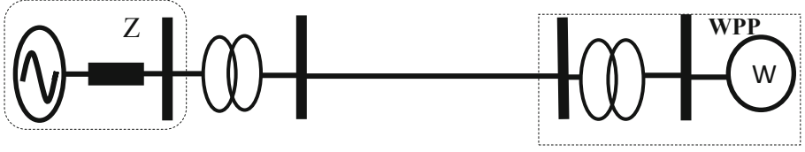
Fig. 2. Single turbine representation of WPP
