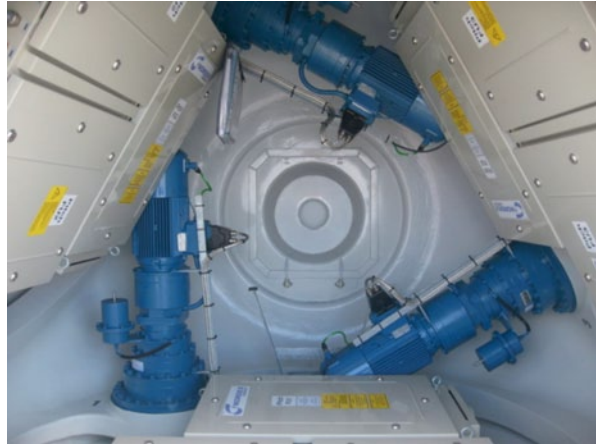
Fig. 2.6 Electric pitch system. (Courtesy of geograph.org.uk (Anderson, Interior of the hub of Turbine No 3, 2008b). © Copyright Paul Anderson and licensed for reuse under this Creative Commons Licence)
