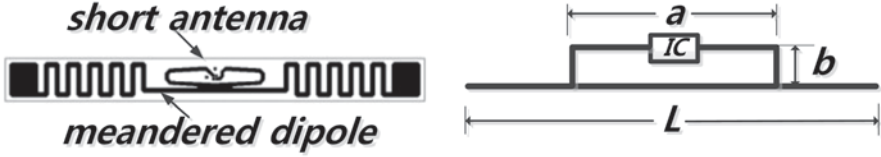
Fig. 2.6 Real tag model and T-match structure
