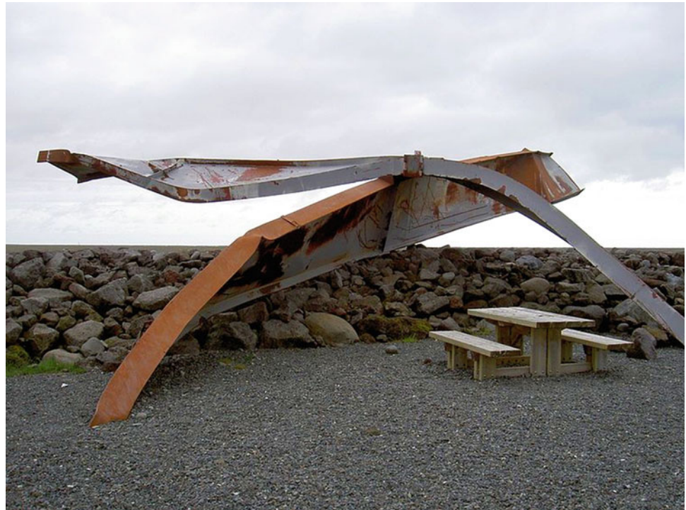
Fig. 2.3 Twisted metal debris from a bridge destroyed by the jökulhlaup produced from the 1996 Gjalp eruption near Grímsvötn. Photo Deanne Bird
