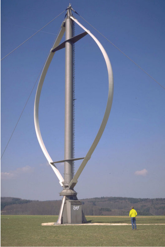
Fig. 2.9 Dornier's Eole-D, height = 20 m, P_{\text{rated}} = 50 kW. Reproduced by permission of EnBW Windkraftprojekte GmbH, Stuttgart, Germany
