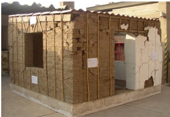
Fig. 28 External cane-rope mesh reinforcement [80]
