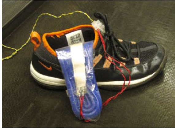
Fig. 2.22 Prototype of the piezoelectric film energy harvesting device inserted in a shoe. There are two DT4-028 K/L piezoelectric films from MSIUSA in parallel inside the shoe. Reproduced with permission from [82]. Copyright @ 2006, Elsevier
