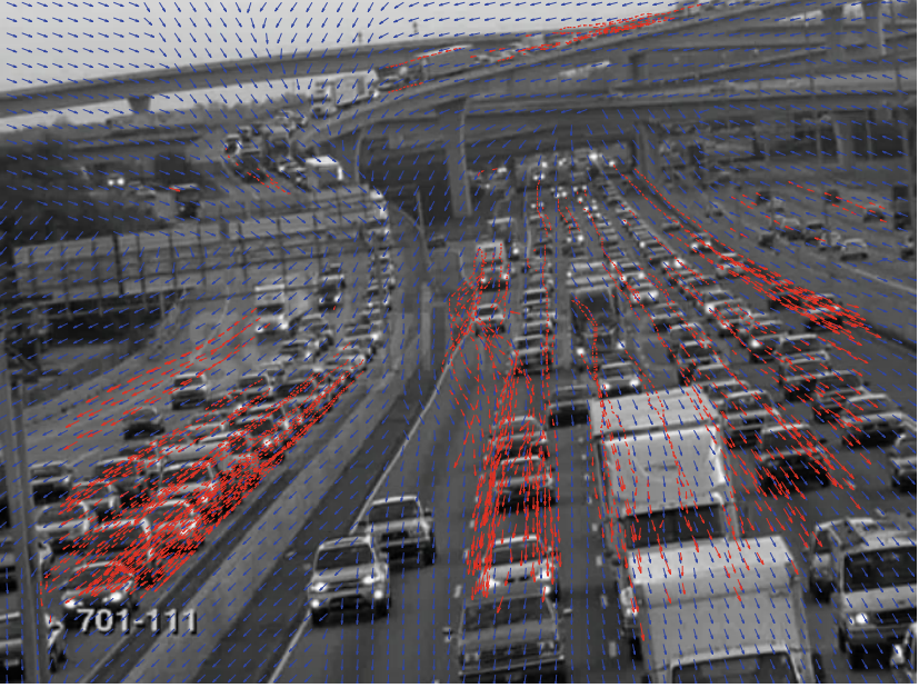
Fig. 3. Regularization of principal motion directions. The red arrows demonstrate measurements of motion cues based on a normalized cross-correlation tracker. Blue arrows demonstrate the regularized directions fields.
