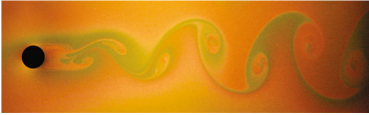
Fig. 2.6 The wake structure of a cylinder in a flowing soap film. The Re number in the experiment is 300
