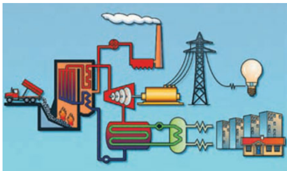
Fig. 2.134 Work schematic for Sysav garbage power plant
