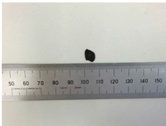
Fig. 2.12 CuNPore (cat-3) size: 175 \mu\text{m} (thickness) \times 5 mm \times 5 mm
