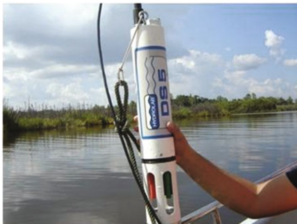
Fig. 2.30 Surveying of Bera Lake water qualities by Hydrolab DS5 apparatus
