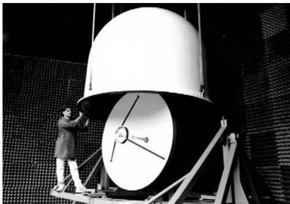
Fig. 1 Installation of radome over the antenna
