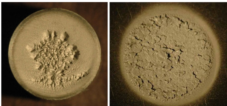
Fig. 2.3 Aluminum alloy Al 7075 samples tested at DYNAFLOW by ASTM G32 direct method ( left ) and alternative method ( right ). Both pictures are shown for 900 min of exposure to cavitation. (Button samples diameter: 12.7 mm)
