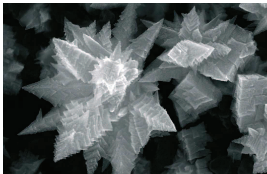
Figure 4.8: Nanostructuring of platinum in the form of nanoparticles. Clef CEA n° 59. Courtesy of CEA. The results have been obtained by the CEA in the framework of a Challenge innovation program.
