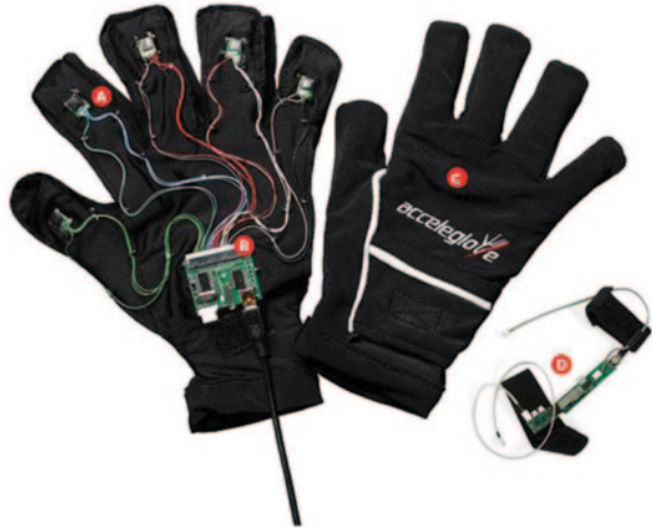
Fig. 2.3 MIT Aceleglove with its multiple sensors. [8]
