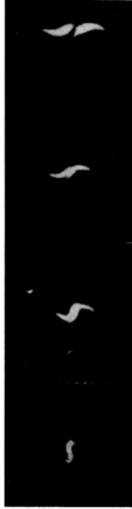
Fig. 2.13 The evolution of two plasmoids fired at each other across a magnetic field (Courtesy W. Bostick)
