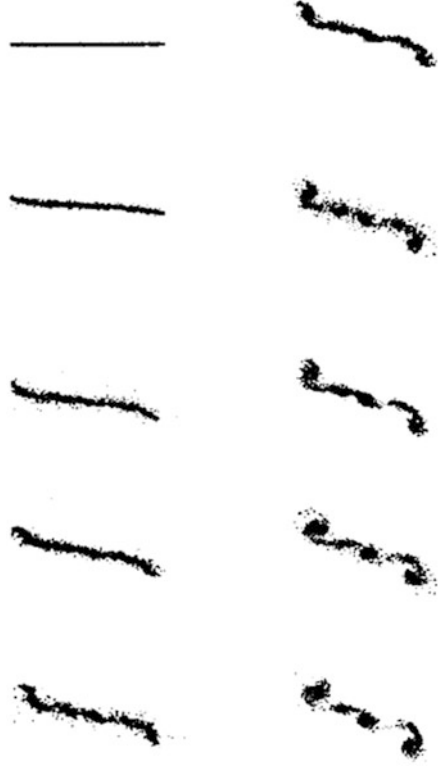
Fig. 2.28 Simulated aurora. Current increases continuously from top to bottom in each column. The simulated beam is analogous to the experimental conditions leading to the data shown in Fig. 2.15
