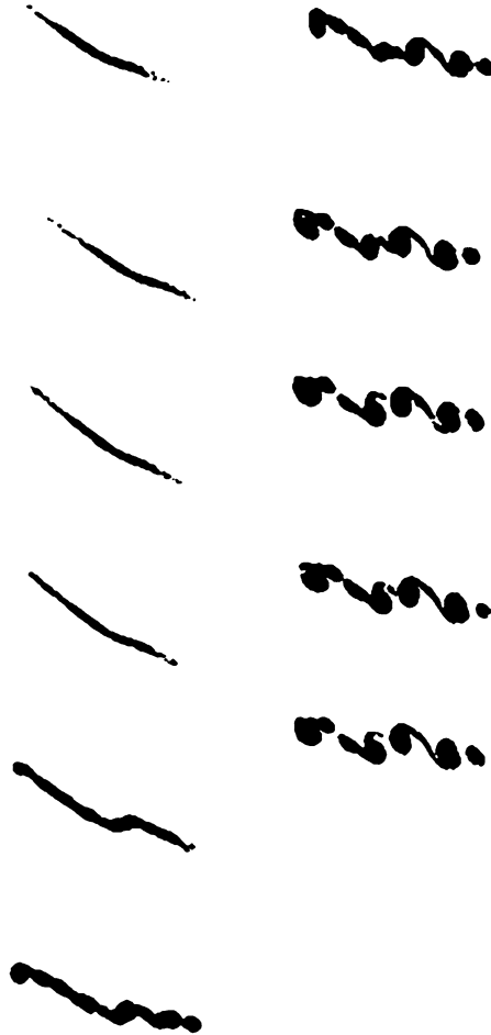
Fig. 2.15 Laboratory simulated aurora. Voltage (current) increases continuously from top to bottom in each column, and the beam pinches only at the edge. In contrast, cold beams with a radius of a few are noncurrent neutralized and exhibit strong pinching
