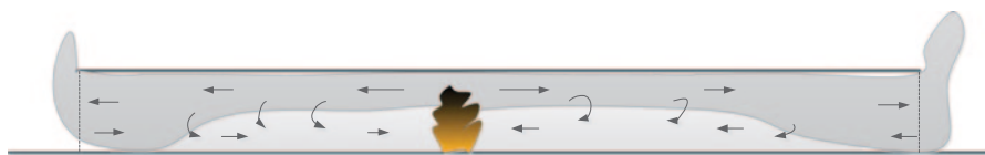
Fig. 2.4 Schematic representation of an inerted fire in a long tunnel. The arrows pointing toward the fire indicate inerted (vitiating) air flow
