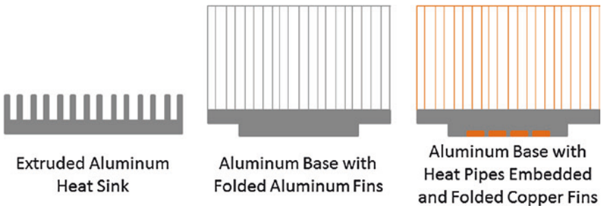
Fig. 2.9 Various heat sink configurations
