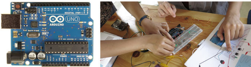
Fig. 2.8 Arduino is an open-source physical computing platform based on a simple microcontroller board and on a system of multimedia programming environment that allows to script and control software for the board. Arduino can be used to develop interactive objects, products and prototypes, since it is able to translate inputs from a variety of switches or sensors into a series of physical outputs controlling lights or motors
