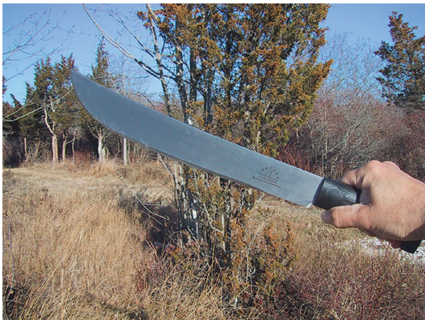
Fig. 2.3 A machete is used for cutting brush when surveying in the woods. Surveyors must be careful not to cut on abutting property without consent of the owner
