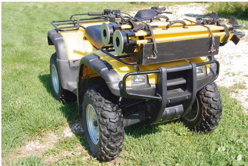
Fig. 2.4 All terrain vehicle (four-wheeler) set up to carry surveying equipment in remote areas or in large acreages. Notice the instrument tripods mounted in a special fixture
