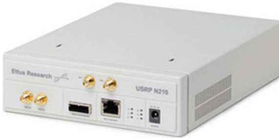
Fig. 2.1 USRP N210—Ettus research. Photo courtesy— https://www.ettus.com/product/details/UN210-KIT
