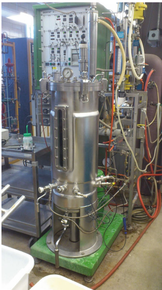
Fig. 2.4 Cultivation of bacteria for biocement production in 50 L fermentor(photo taken at the Fermentation Facility, Iowa State University,USA)
