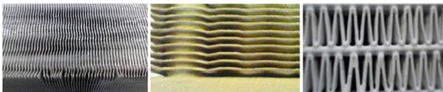
Fig. 2.2 Three examples of dip coated adsorbers, employing a binder: silica gel coating, by Sortech [22], on the left hand side , AQSOA Z01 coating, by Mitsubishi [27], central , SAPO 34 coating, by CNR ITAE and University of Messina [28], on the right hand side
