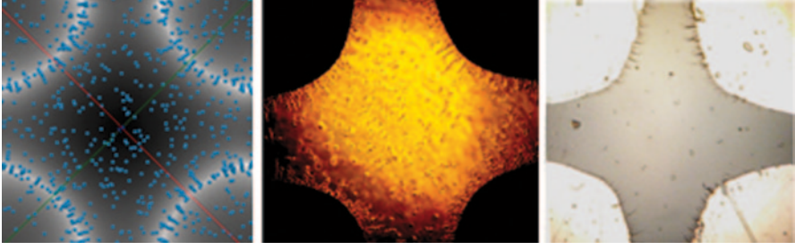
Fig 2.1 Comparison of the top view spatial distributions obtained with simulation and experiments: left ) the Monte Carlo simulation with superimposed the intensity map of the electric field, center ) Distribution of MDA-MB-231 after 180 s of DEP manipulation ( V_{pp}=8V f=1000 kHz), right ) Distribution of MWCNT after 10 min of DEP manipulation ( V_{pp}=80V f=300 kHz)
