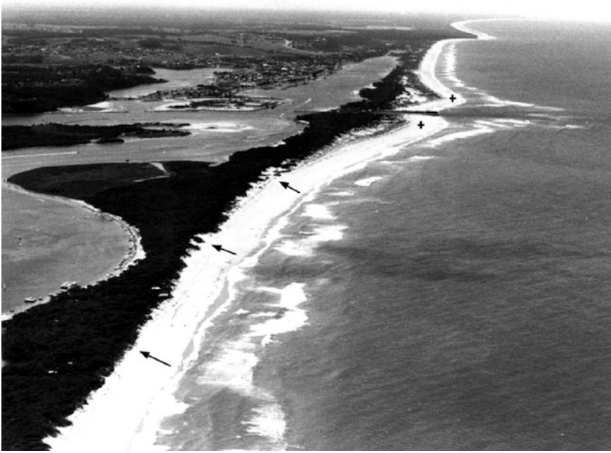
Fig. 2.6 Erosion ( arrowed ) of the Ninety Mile Beach, on the outer barrier of the Gippsland Lakes in SE Australia, with accretion (+) on either side of the Lakes Entrance breakwaters. © Geostudies
