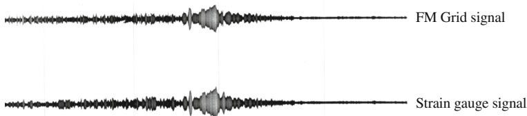
Fig. 5 Visual comparisons of strain gauge and FM grid output
