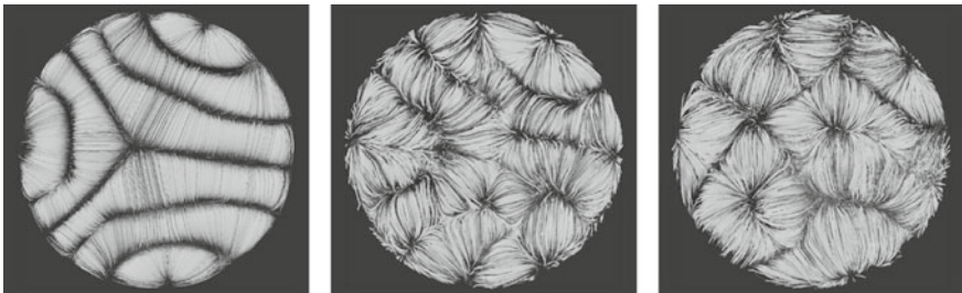
Fig. 5 Images from Bailon-Cuba et al. (2010) showing the polygonal structures of the time-averaged streamlines of the direct numerical simulations in a Rayleigh-Bénard cell with \Gamma = 8 for Ra = 6,000 , 10^7 , and 10^8 , respectively
