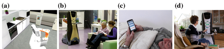
Fig. 4 Evaluation of the user interface for elderly people. a Lab evaluation where robot simulation showed robot actions in modeled home environment. b Evaluation in model kitchen. c and d Evaluation in real homes of elderly people
