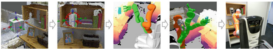
Fig. 10 Interaction sequence for semi-autonomous reaching and grasping of an object unknown to the robot
