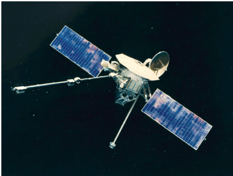
Fig. 2.1 Mariner 10 as it would have looked in flight. Each solar panel was 2.69 m long, and housed three pairs of orthogonal nitrogen gas reaction thrusters to control and stabilize the spacecraft's attitude. The arm extending to the left is the magnetometer boom, which was 5.8 m long. The flat white dish is the sunshade, through which the main engine's nozzle (invisible) projected. The steerable high-gain antenna for communications sticks out beyond the sunshade. The shorter arm houses the omnidirectional low gain antenna (NASA)
