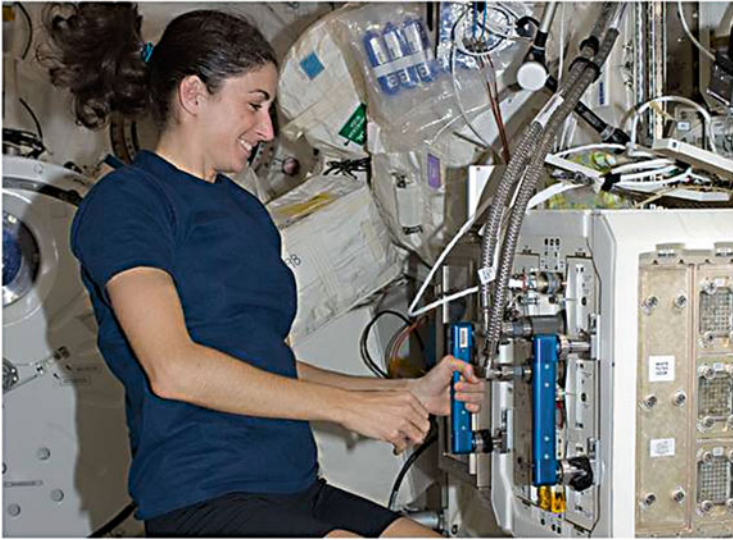
Fig. 2.10 The 91 days duration mice drawer system (MDS) module scenario (Aug 28 to Nov 27, 2009, STS 128/129, PI Cancedda) on the International Space Station (ISS). NASA Astronaut Nicole Scott onboard the ISS at the Japanese Kibo Laboratory with the MDS module (right side) housing three ( n = 3 ) C57Bl/10 J and three ( n = 3 ) osf-1 transgenic mice (Courtesy: NASA ( http://onorbit.com/node/1601 ))
