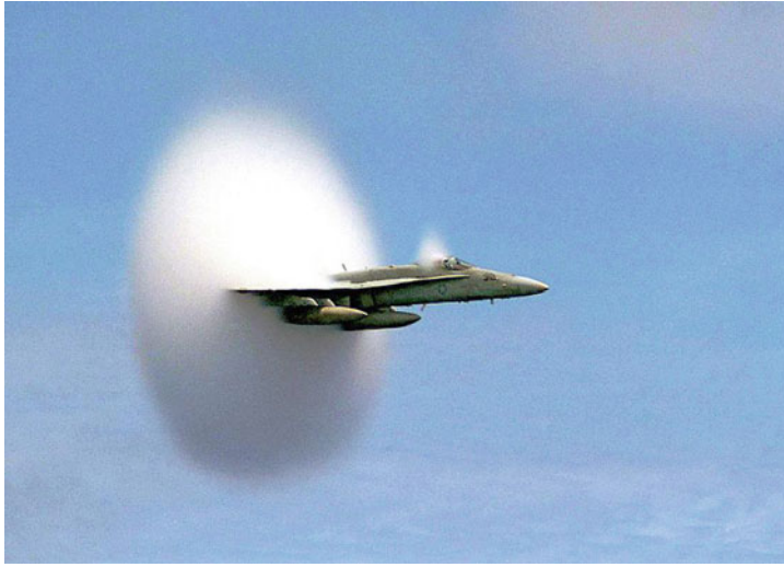
Fig. 2.4 An F/A-18 Hornet creating a vapor cone at transonic speed just before reaching the speed of sound (7_July_1999)
