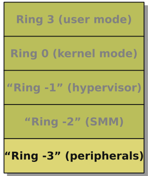
Fig. 2.1 “Ring -3” environment compared to other rootkit environments on the x86 platform. Please note, ring 3 and ring 0 are implemented in hardware (host CPU). The terms “ring -1”, “ring -2”, and “ring -3” are used to emphasize the power of the corresponding execution environments. They are not implemented in hardware
