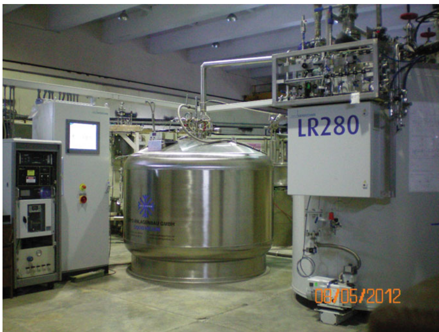
Fig. 1.8 A modern day turbine based helium liquefier with a refrigeration capacity of 900 W ( \sim 300 l/h) manufactured by Linde Kryotechnik AG installed at IUAC in 2012 (Photo courtesy IUAC Delhi)
