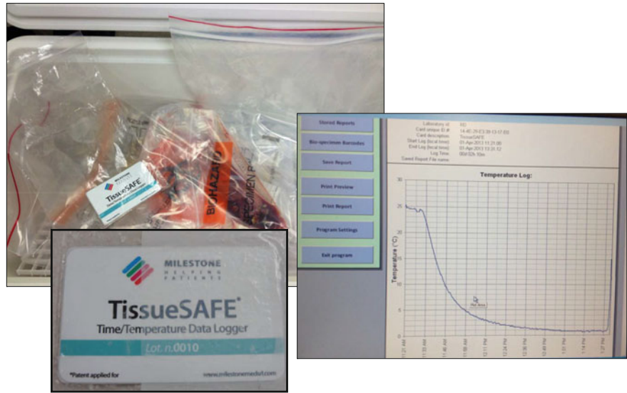
Fig. 5 RFID card records the run temperature
