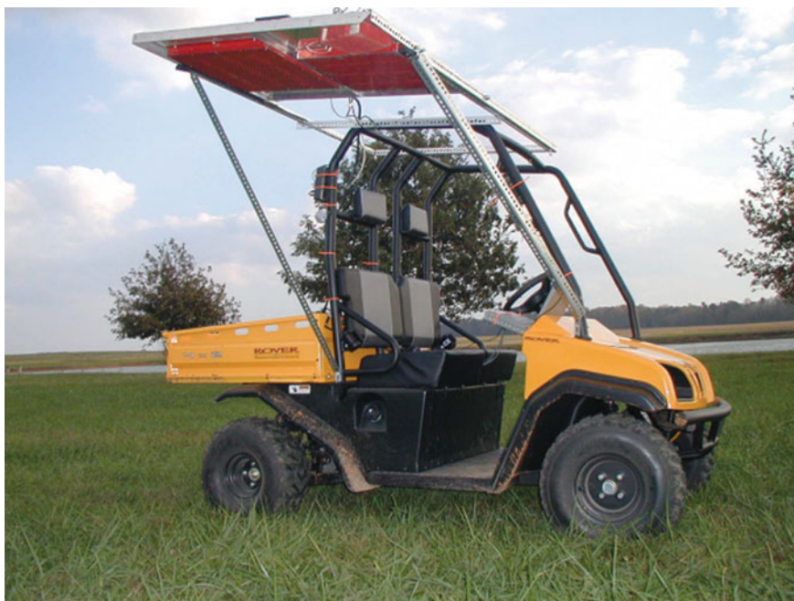
Fig. 2.8 General view of the manned “Rover” type mobile platform equipped with three portable microwave radiometers, operating at the wavelengths 6, 18, and 21 cm. Also equipped with a folding panel of 1.5 \text{ m} \times 1.5 \text{ m} for instrumentation installation along with GPS receiver, data acquisition system and power supply battery (Shutko et al. 2010; Krapivin and Shutko 2012; Verba et al. 2014)
