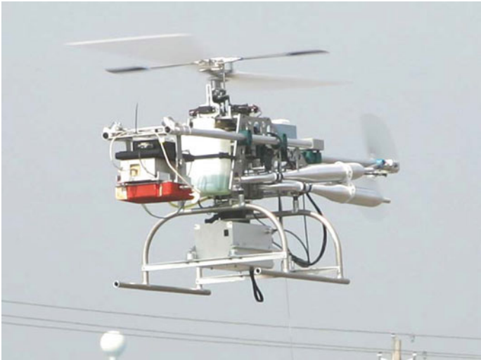
Fig. 2.10 Photograph of the unmanned aerial vehicle (UAV) helicopter “Microwave Autonomous Copter System” (MACS) equipped with a 6 cm radiometer, data acquisition system, GPS receiver and power supply battery (Shutko et al. 2010)
