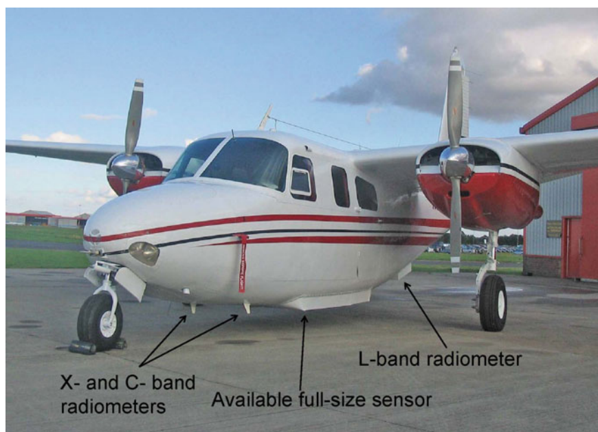
Fig. 2.7 Miramap sensor aircraft (Shutko et al. 2010; Krapivin and Shutko 2012)
