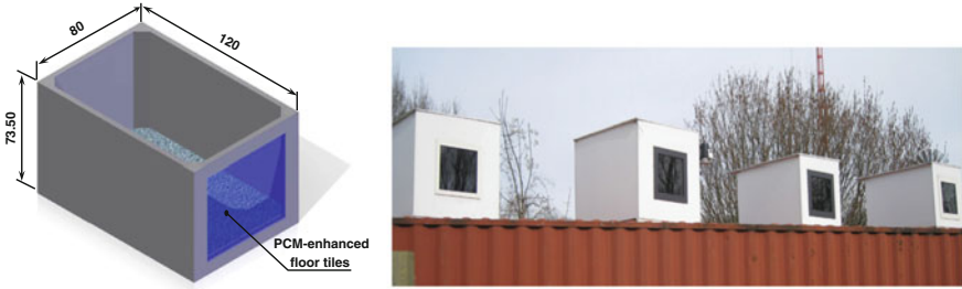
Fig. 2.9 Test containers used by University of Twente, the Netherlands, to test PCM floor tiles. Entrop et al. (2011)
