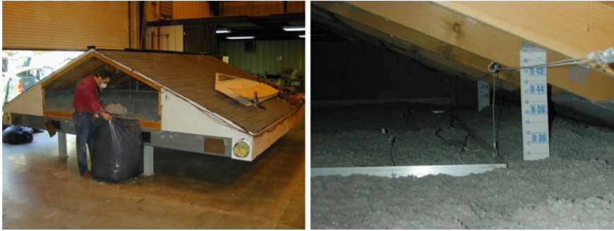
Fig. 2.17 Experimental attic module containing microencapsulated PCM blended with cellulose insulation, ORNL, USA, testing facility
