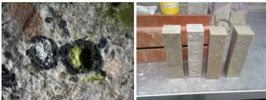
Fig. 2.2 Microscopic view of the concrete— inorganic PCM mixture (left) and test samples of PCM—enhanced concrete (right) (van Haaren 2012)
