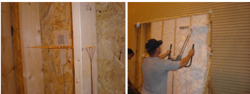
Fig. 2.8 Installation of the test wall containing PCM-enhanced fiberglass insulation. Left side presents wall cavity instrumentation with array of thermocouples installed across the wall cavity. Right side Cavity finish task, after blowing in fiberglass insulation
