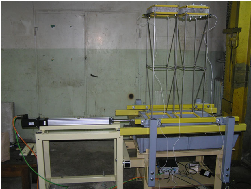
Fig. 2.10 Setup of the shaking table experiment
