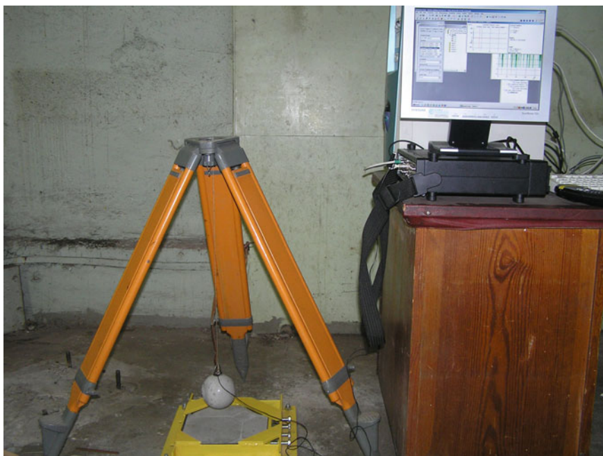
Fig. 2.5 Setup of the impact experiment
