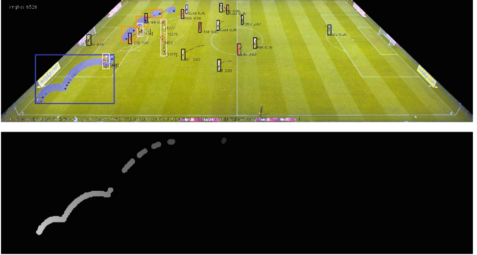
Fig. 2. Sample snapshot of the processed input image sequence including detected ball tracklets marked by rectangles (top) and one for the corresponding motion history image (bottom).
