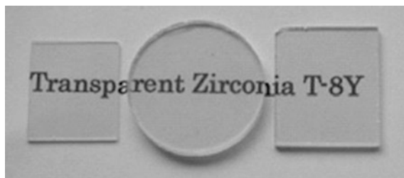
Fig. 2.3 Photographs of representative YZS transparent ceramics, which were made from commercial powder with hot isostatic pressing sintering method. Reproduced with permission from [88]. Copyright © 2008, John Wiley & Sons
