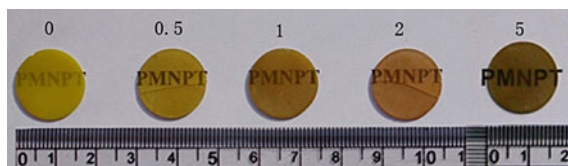
Fig. 2.21 Photographs of the \text{Er}^{3+} -doped PMN-0.25PT transparent ceramics with a thickness of 1.5 mm. The numbers in the photographs are the \text{Er}^{3+} doping levels in mol%. Reproduced with permission from [237]. Copyright © 2012, Elsevier
