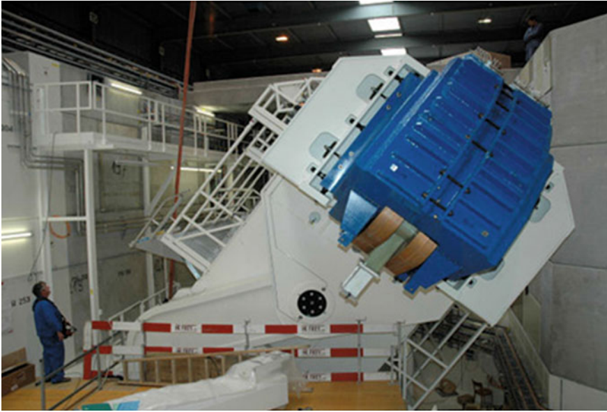
Fig. 2.16 The gantry mechanism and final dipole of Gantry 2 at the Paul Scherrer Institute. The upstream design enables parallel scanning, which thereby simplifies treatment planning and gives an infinite SAD, which assists in skin sparing but necessitates a rather large 45-ton final dipole to give sufficient aperture to deliver the desired treatment field size. Courtesy Prof. Tony Lomax/PSI
