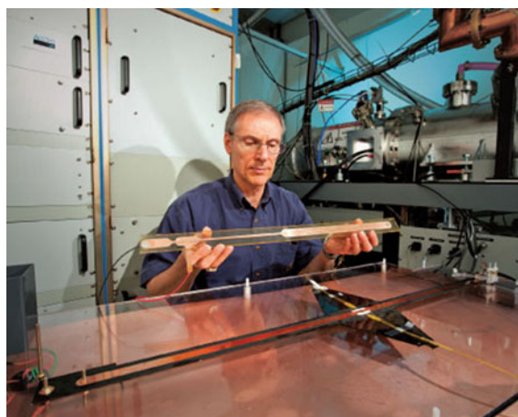
Fig. 2.21 George J. Caporaso examines the Compact Particle Acceleration Corporation's (CPAC's) newest Blumlein design. Tests at the CPAC are combined with computer simulations at Livermore Laboratory to produce a practical design. Courtesy George J. Caporaso
