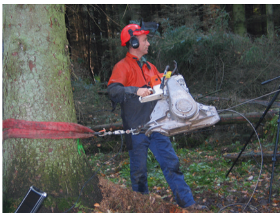
Fig. 2.6 Static tree-pulling with motorized winch to determine critical turning moment (photo credit J.-C. Ruel)
