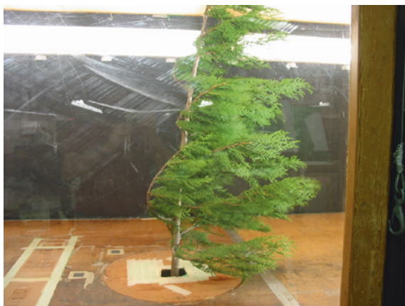
Fig. 2.7 Side view of western redcedar ( Thuja plicata Donn ex D. Don) tree crown in a wind tunnel in horizontal airflow (photo credit S.J. Mitchell)
