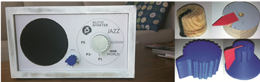
Fig. 2. The PiRadio (left) and the prototypes for the knob (right).
