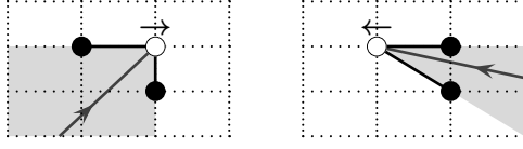
Figure 14: The two modes of operation of the BTBS scheme in Exercise 12.23 with target points ( \circ ). Both modes are stable provided that the characteristics lie in the shaded regions.
