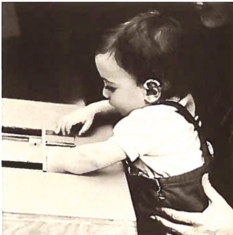
Fig. 16 Two-handed obstacle box for studying the complementary role of right and left hands
