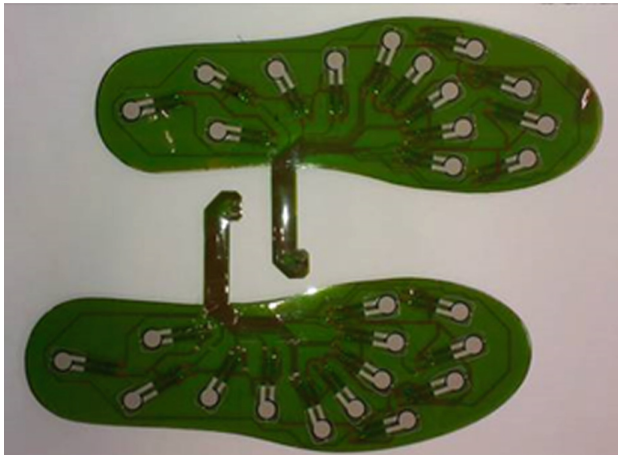
Fig. 2. Pressure sensor layer of the insoles
