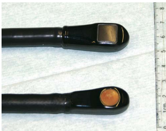
Fig. 2.14 Side-by-side illustration of a transesophageal live 3D matrix array probe with 2600 elements (top; Model x7-2t, 2–7 MHz, Philips Medical Systems, USA) and a standard multiplane 2D phased array probe with 64 elements (bottom; Model Omni 3, Philips Medical Systems, USA)
