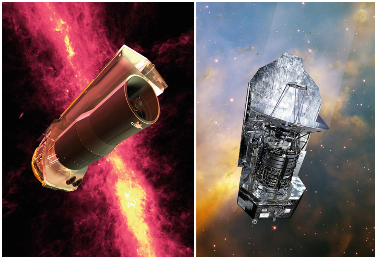
Fig. 1.33 Left: The Spitzer Space Telescope, launched in 2003. Right: The Herschel Space Observatory, launched in 2009 together with the Planck satellite. Herschel is equipped with a 3.5-m mir-
