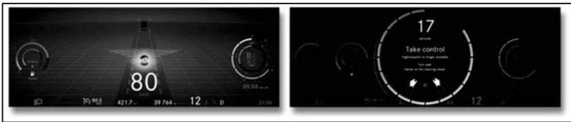
Fig. 1: Instrument display in the Highway Pilot mode and the instruction to the driver to take over control later on
